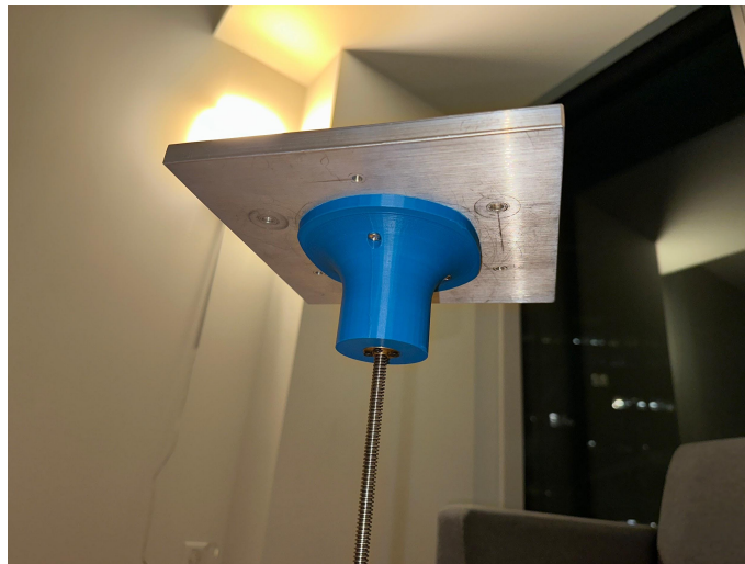
Figure 2.2.3: Printed and Assembled Motor-Plate Connection
