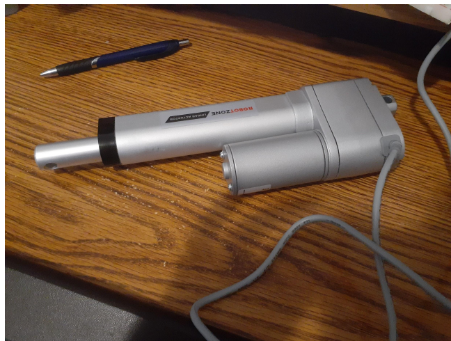
Figure 2.4.2: The linear actuator used in the electromechanical prototype is shown.
